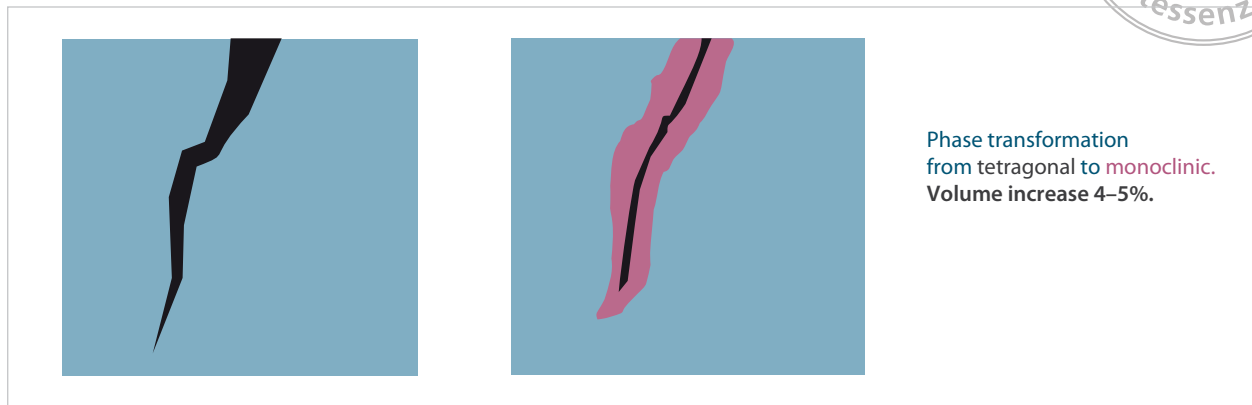
Fig 6 The behavior of zirconia at crack edges.
