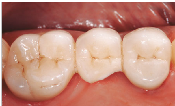
Fig 13 Chipping in veneering ceramic (Initial Zr, GC) on the second premolar of a three-unit zirconia fixed partial denture after 12 months of clinical use.
